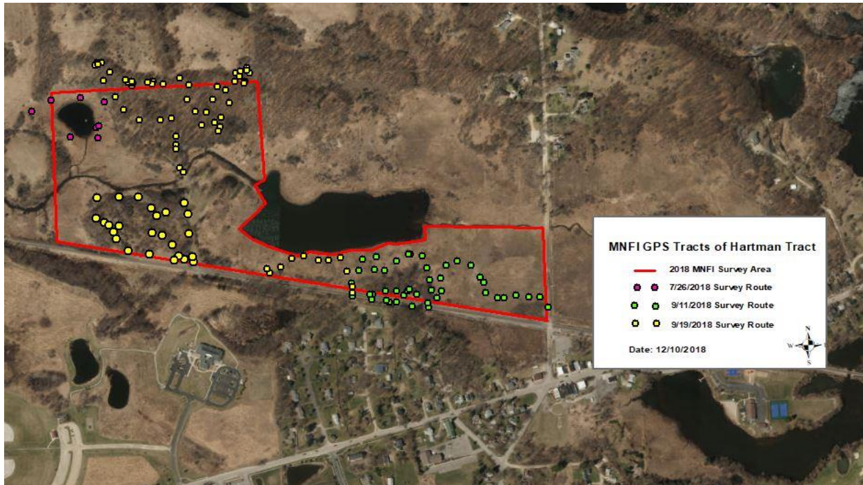
Figure 4. Selected GPS survey routes to show examples of meander-searches; a Garmin Montana model 650t PS unit was employed to record survey tracks for most meander-searches carried out in addition to taking point locations where needed. The map does not depict all survey track routes.
